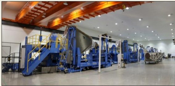
Advanced composite structures are manufactured using automated fiber placement technology on fiber placement machines.
