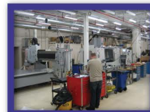
Precision Machine Shop: Gantry Router (5' x 10' Table); 5 Axis Mill (64" x 24" x 24"); Tool Room; Lathe; Support Equipment
