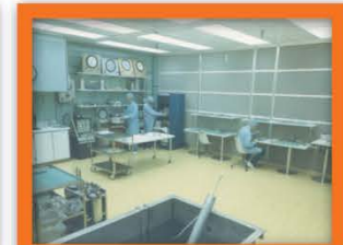
Multiple Clean Rooms/Tents From Class 1k to 100; Largest Has 960 ft 2 Area; Laminar Flow Benches and Orbital Welding and Fab
