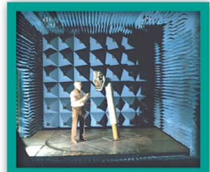
Far Field Range: 704 ft 2 Chamber; 5 ft Diameter Spherical Quiet Zone; 100dB Attenuation From 50MHz -100GHz Frequencies; 150dB Isolation
