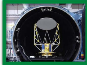
3 Large TVAC Chambers (10-7 Torr) (Largest is 18ft Diameter/32ft Length). Multiple Smaller Chambers for Electronics Boxes and Piece Part Bakeouts
