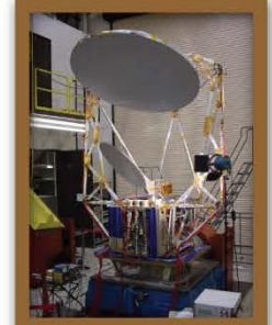
Vibration Facilities Has Shakers From 1klbs to 50klbs for Vertical and Horizontal Modes
