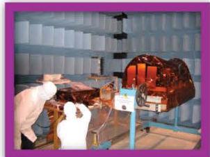
EMI/EMC Test Facility: 100dB Attenuation From 10kHz to 20 GHz; Standard and Non-Standard (Single Event Switching Transients; Abnormal Voltage, Surge Voltage) Capabilities
