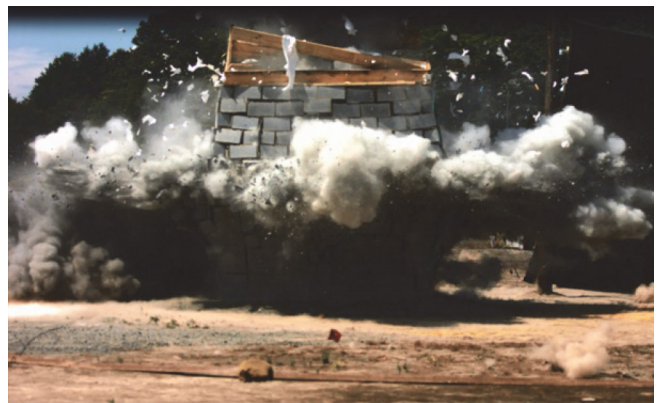
Figure 3. Concrete masonry unit for characterizing building debris
