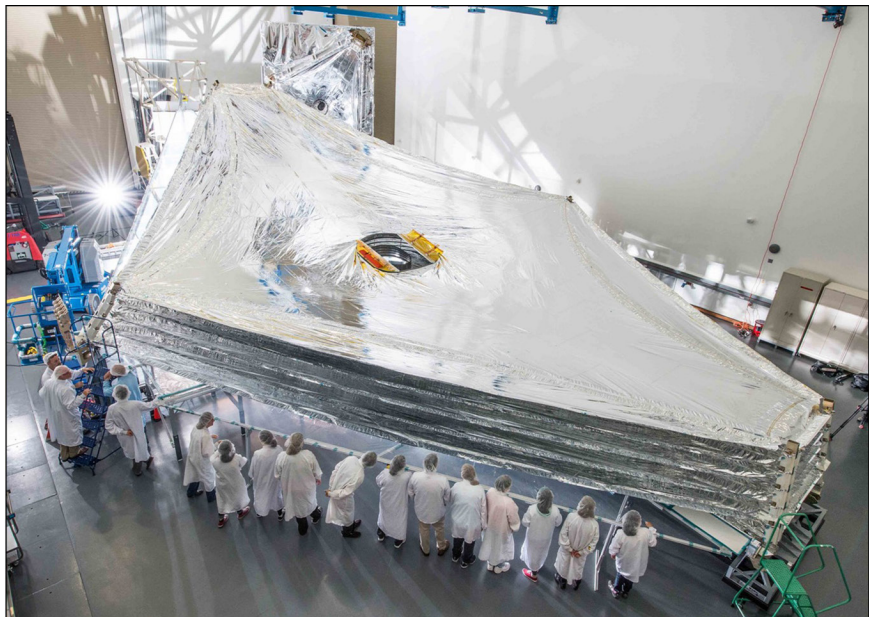
Figure 6: James Webb Space Telescope's Sunshield Template Layers
