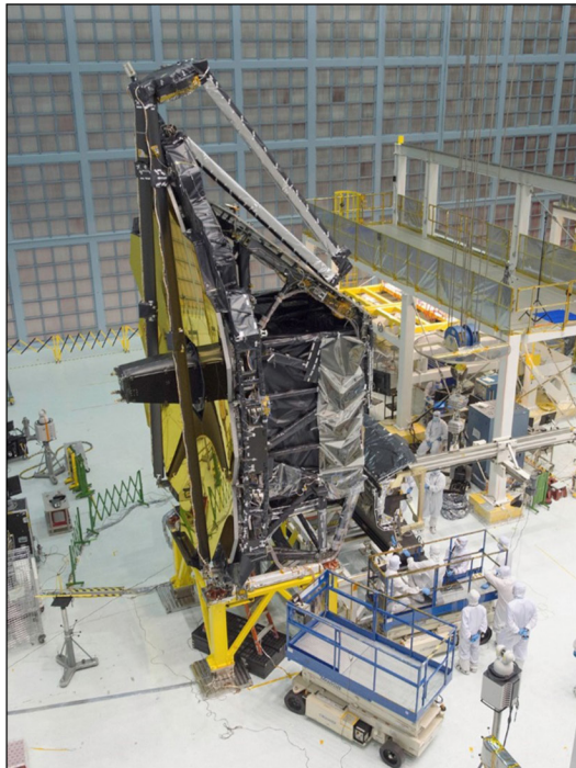
Figure 4: James Webb Space Telescope's Optical Telescope Element and Integrated Science Instrument Module
