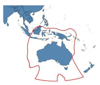
Example coverage of Asia from a satellite located at  $135^{\circ}$  East Longitude
