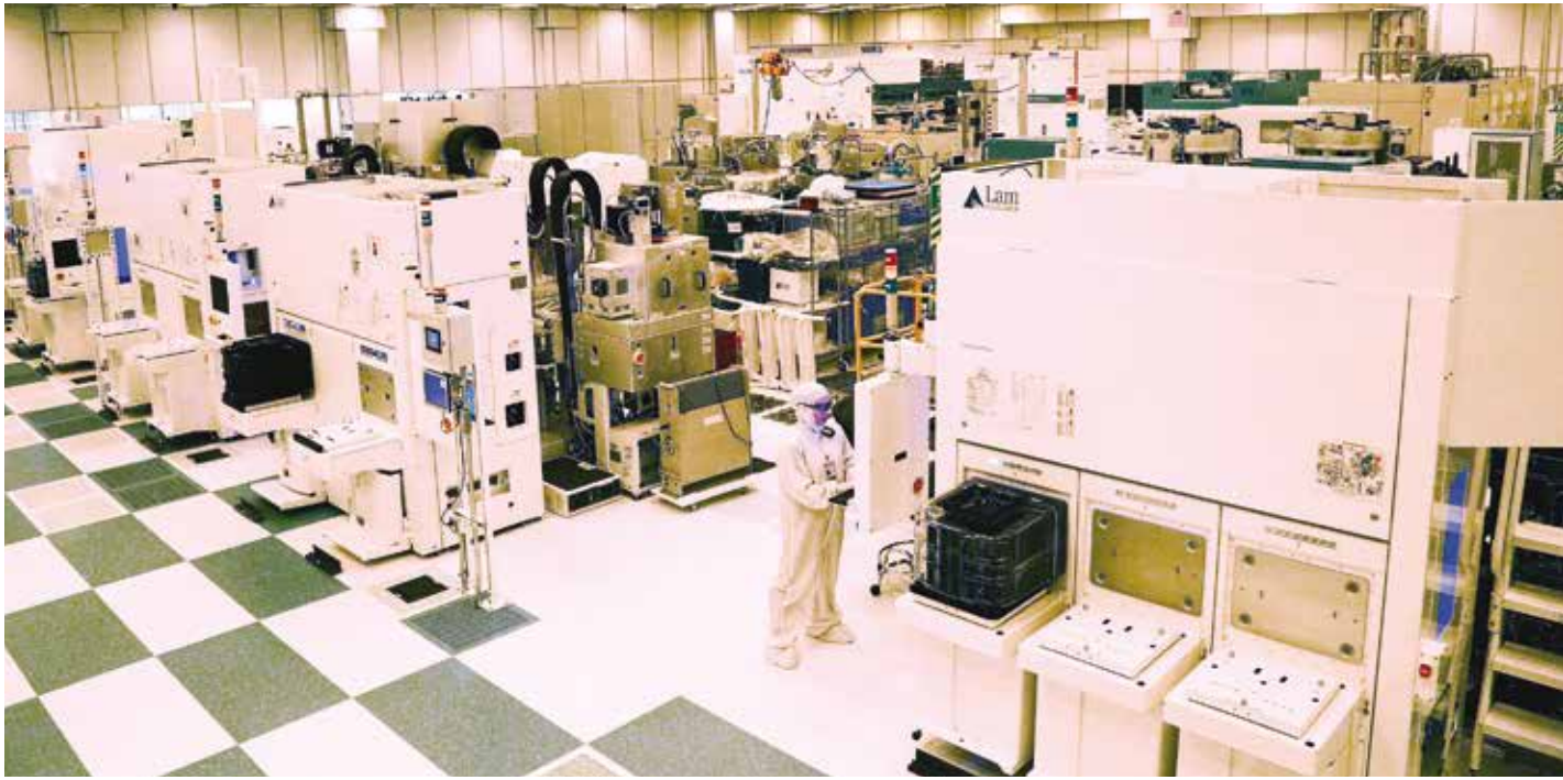
The clean room used to manufacture the integrated photonic circuits that the American Institute for Manufacturing (AIM) will be providing future access to through multiproject silicon wafer production runs.
