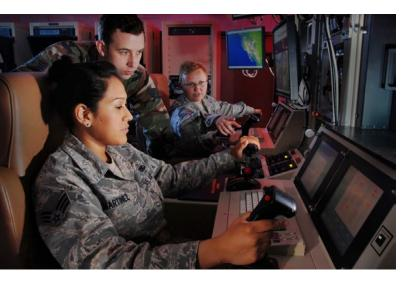
U.S. Airmen from the 163rd Maintenance Group, which is a part of the California Air National Guard and primarily involved in the Predator missions, train on a ground control station. The Predator drone runs on the open source operating system Linux. (Val Gempis/U.S. Air Force)
