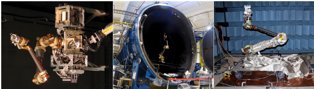
Figure 3-2. FRENDS Flight Prototype, Functional and Environmental Testing
