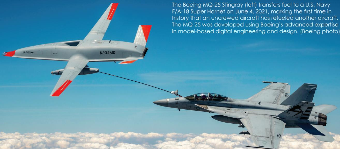
The Boeing MQ-25 Stingray (left) transfers fuel to a U.S. Navy F/A-18 Super Hornet on June 4, 2021, marking the first time in history that an uncrewed aircraft has refueled another aircraft. The MQ-25 was developed using Boeing’s advanced expertise in model-based digital engineering and design. (Boeing photo)
