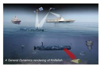
The Knifefish unmanned underwater vehicle designed for hunting mines as part of the mine countermeasures mission module for the Navy's Littoral Combat Ships is scheduled for a first round of sea testing this summer.
